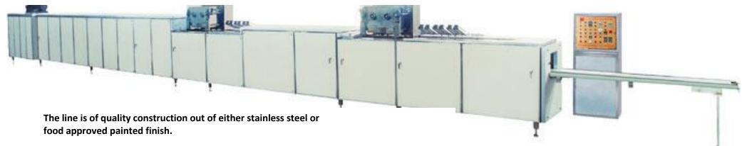
The machine has all the parts required for a modern day moulding machine, this includes chain secured moulds, mould heating, one shot depositing, vibration, refrigerated cooling and de moulding. We can also supply depositing heads that will produce a two colour outer shell.
