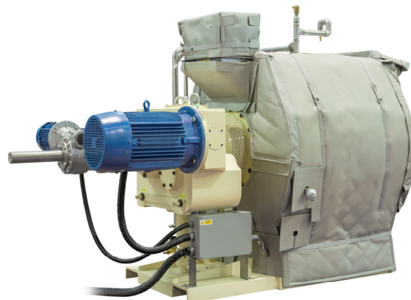
*Conche fitted with Noise Reduction Blanket
